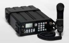
The Codan 2110v Manpack suits voice only operations, providing a cost effective, reliable and rugged portable communications solution. Available with FED-STD-1045 ALE for automated channel selection and linking, and secure voice modes, the Codan 2110v Manpack is a smart choice for highly portable long distance voice communications.
